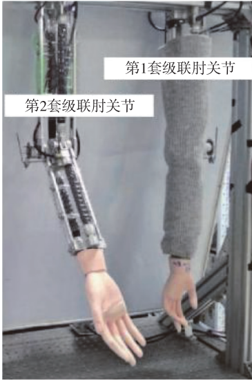
图 12 气动肌肉仿生肘关节 [39] Fig. 12 Pneumatic muscle bionic elbow joint [39]
