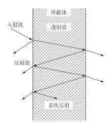
图 1 屏蔽机理示意 Fig. 1 Shielding mechanism scheme
