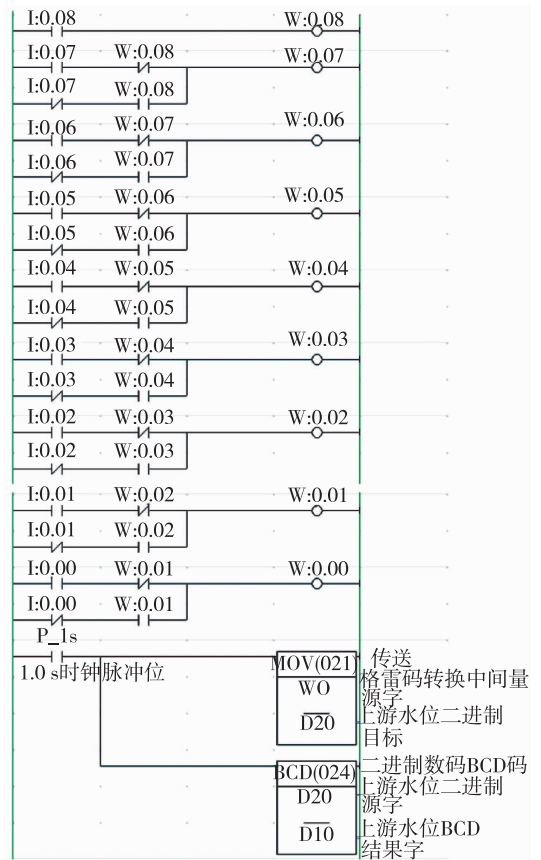
图4 上游水位的采集程序 Fig.4 The data acquisition program of upstream level
