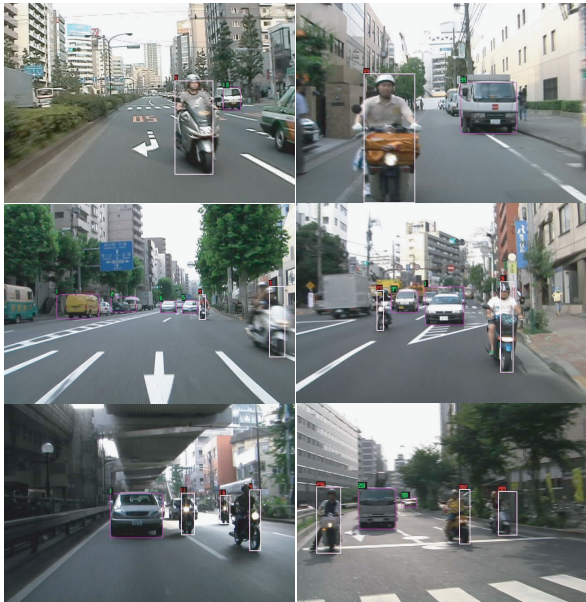
图 4 不同数量摩托车被成功检测的例子 (白色矩形框表示识别的摩托车) Fig. 4 Examples of successful detection by the proposed method (white bounding-boxes referring to the detected motorcycles)
